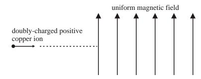
The diagram above shows a doubly-charged positive ion of the copper isotope  $^{63}_{29}$ Cu that is projected into a vertical magnetic field of flux density 0.28 T, with the field directed upwards. The ion enters the field at a speed of 7.8 × 10<sup>5</sup> m s<sup>-1</sup>.
