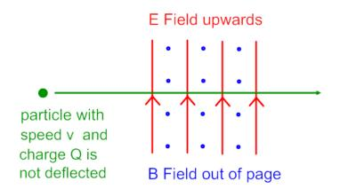
Find an expression for this velocity, v, in terms of the electric field strength E and magnetic field strength B. Show that v does not depend on the charge, Q, of the particle.
